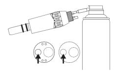
Use "Safco Handpiece Premium Service Oil (102-3700)" for care and lubrication. Remove the Air Motor from the tubing, attach the enclosed Vector oil adapter on the oil can and spray for 1-2 seconds in the smaller one of the two large pipelines (see drawing).
